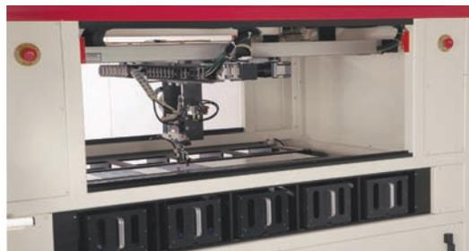
Tested cells are sorted into output bins according to the cell's electrical performance.
