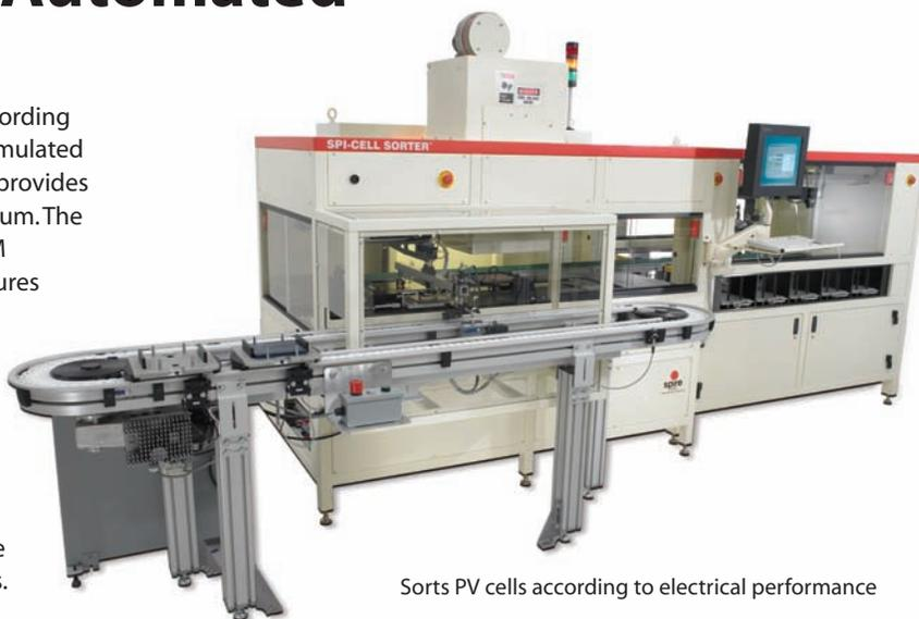
Sorts PV cells according to electrical performance
